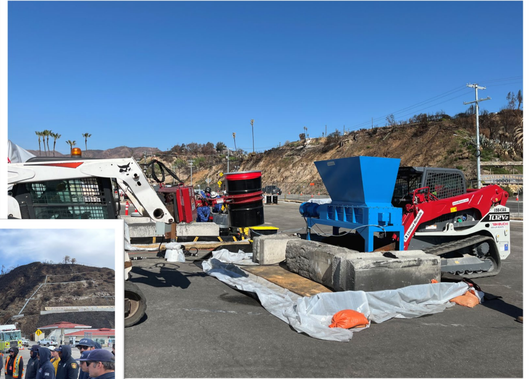
First time a battery shredder was deployed to process batteries in the field
