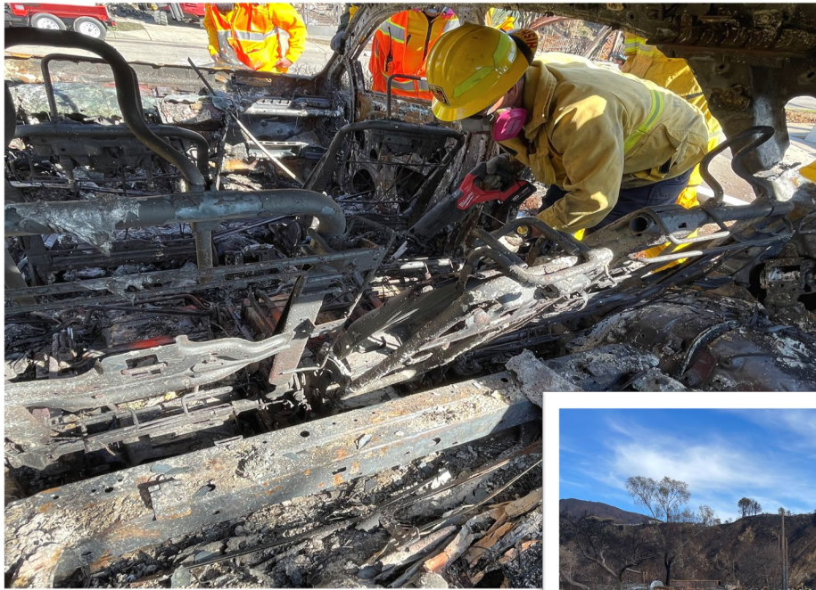
LA City's OES HM12 removing a battery from a hybrid vehicle
